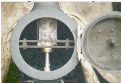
***Type 3 – Internal Mesh Arrestor***
